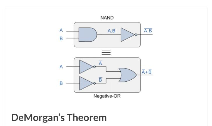
DeMorgan's Theorem and Laws can be used to to find the equivalency of the NAND and NOR gates
