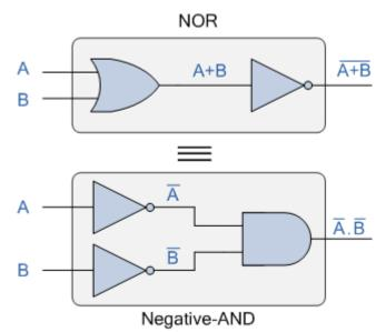
The top logic gate arrangement of:  $\overline{A+B}$  can be implemented using a NOR gate with inputs A and B. The lower logic gate arrangement first inverts the two inputs producing  $\overline{A}$  and  $\overline{B}$  which become the inputs to the AND gate. Therefore the output from the AND gate becomes:  $\overline{A}.\overline{B}$
