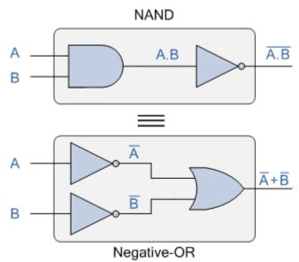
The top logic gate arrangement of:  $\overline{A.B}$  can be implemented using a NAND gate with inputs A and B. The lower logic gate arrangement first inverts the two inputs producing  $\overline{A}$  and  $\overline{B}$  which become the inputs to the OR gate. Therefore the output from the OR gate becomes:  $\overline{A}+\overline{B}$
